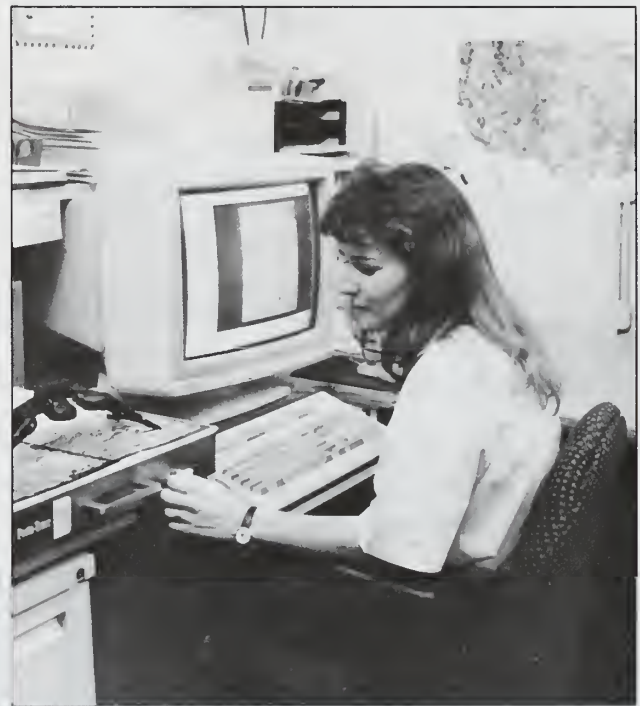
Figure 13. USGS digital superpositioning system workstation operation using commercial GIS software for Digital Line Graphic (DLG) production.
